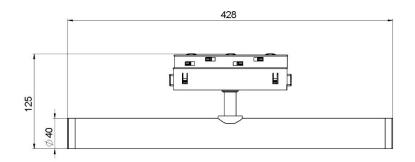
Dimensions: 428 x Ø40 x 125mm Total power: 10 w Luminaire luminous flux: 1000 lm Luminaire efficacy: 100 lm/w Weight: 0.45 kg
